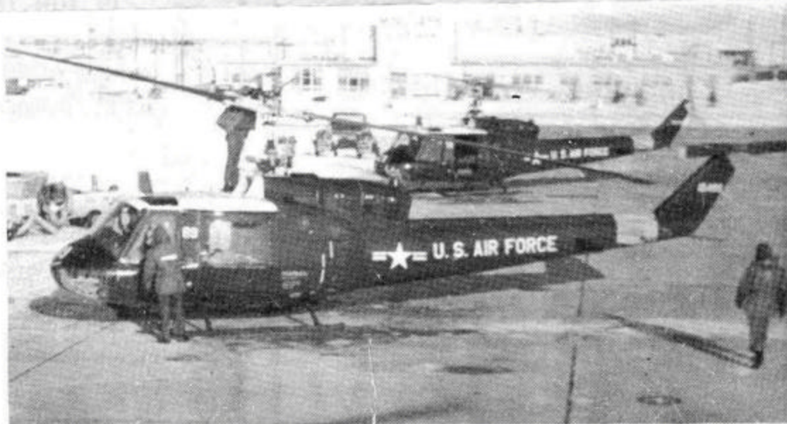
PRE-FLIGHT INSPECTION — Maintenance personnel perform a pre-flight inspection on a Bell UH-1F Iroquois helicopter. The helicopter carries personnel and supplies to various missile sites. (U.S. Air Force Photo)
