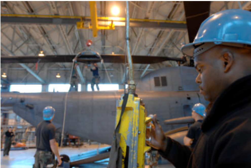
Manning the overhead hoist, Tech. Sgt. Michael Barns, an avionics specialist assigned to the 352nd Maintenance Squadron, Helicopter Maintenance Unit, RAF Mildenhall, England, works closely with two other team members positioned on the tail section of one of five MH-53M Pave Low IV Helicopters assigned to the 21st Special Operations Squadron, to gently lift each blade to remove tension before the eight bolts that hold it in-place can be removed, Oct. 02, 2007.
