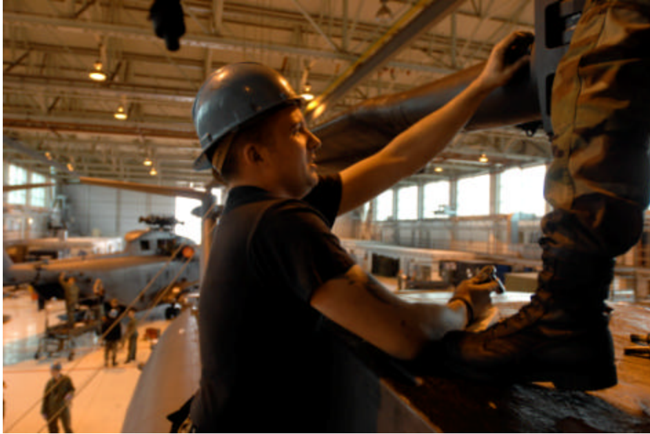
Crew chief, Airman 1st Class Chris Ollivier, from the 352nd Maintenance Squadron, Helicopter Maintenance Unit, RAF Mildenhall, England, removes one of eight bolts holding a 350 pound rotor blade from one of five MH-53M Pave Low IV Helicopters assigned to the 21st Special Operations Squadron, Oct. 02, 2007.
