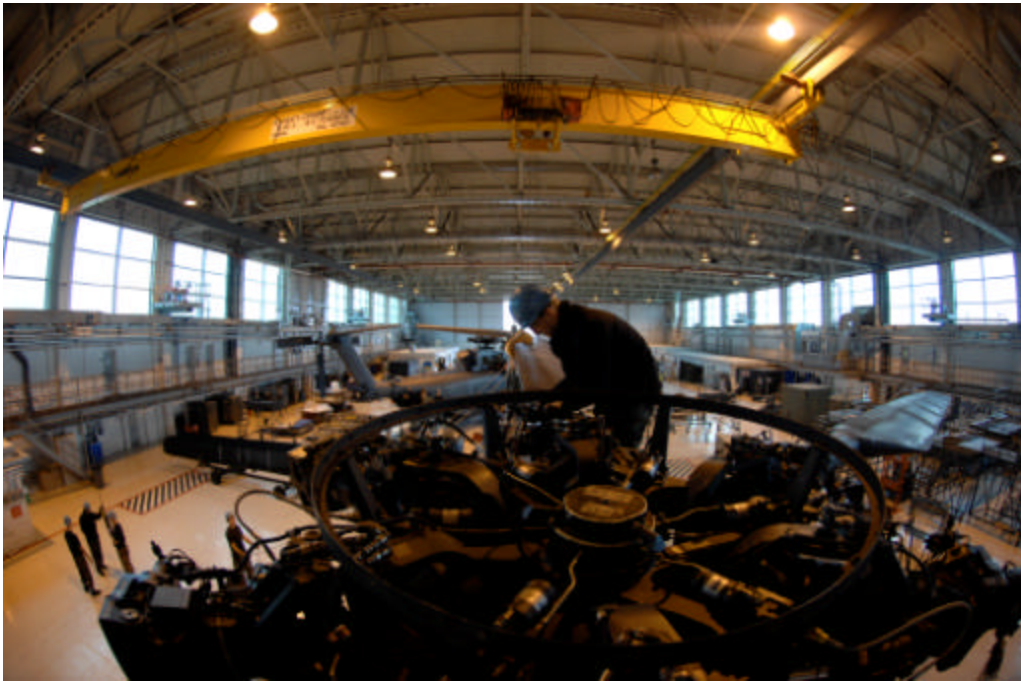
Positioned near the rotor head on top of one of five MH-53M Pave Low IV Helicopters assigned to the 21st Special Operations Squadron, Senior Airman Brad Renninger, a crew chief in the 352nd Maintenance Squadron, removes bolts that hold the rotor blades in place, Oct. 02, 2007, RAF Mildenhall, England.
