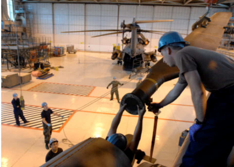
Staff Sgt. Justin Rich, a crew chief from the 352nd Maintenance Squadron, Helicopter Maintenance Unit, guides the last rotor blade away from MH-53M Pave Low IV tail number 95784 during the dismantling process to prepare the aircraft for storage at the Aerospace Maintenance and Regeneration Group in Tucson, Ariz., commonly known as the 'Boneyard,' Oct. 02, 2007, RAF Mildenhall, England. Each rotor blade weighs 350 pounds and is lowered to the ground using an overhead hoist.
