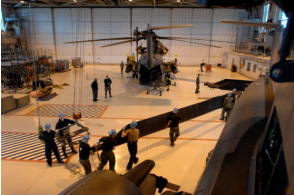
Crew chiefs and aircraft specialists in the 352nd Maintenance Squadron, Helicopter Maintenance Unit, remove rotor blades from one of the five MH-53M Pave Low IV Helicopters assigned to the 21st Special Operations Squadron, RAF Mildenhall, England, Oct. 02, 2007.
