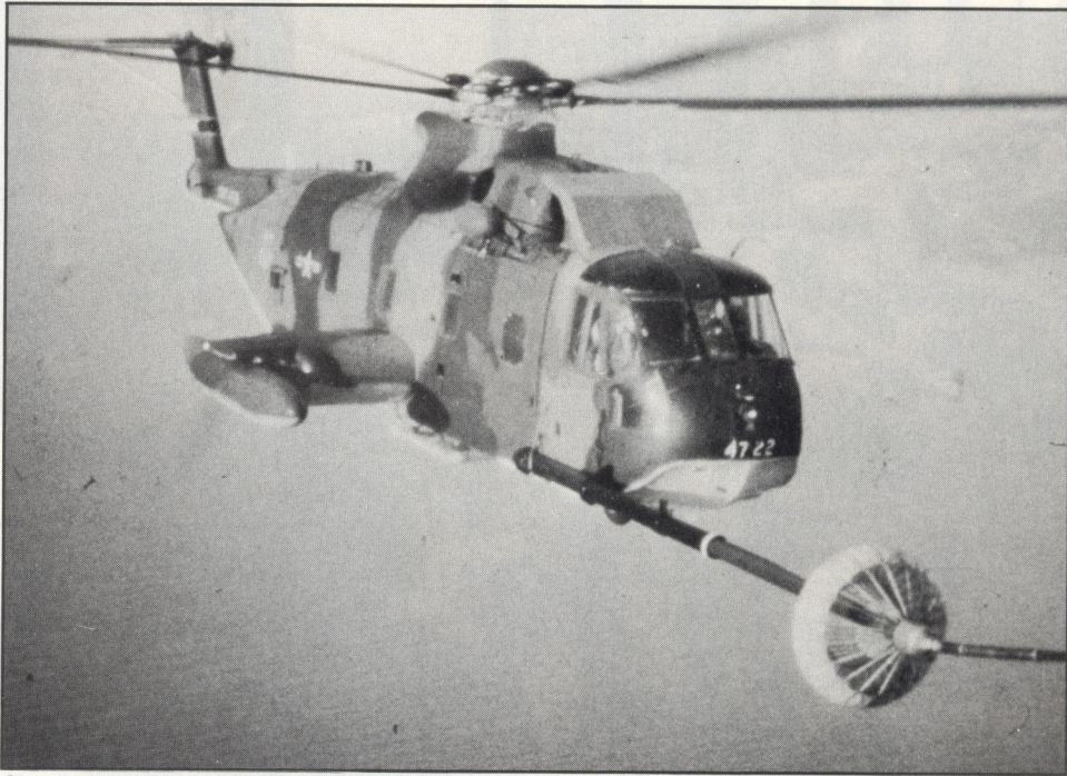
Close-up of the HH-3E in the process of refueling in flight (aerial replenishment procedures with tankers and helicopters were first established in 1965). This was a demanding task — even more difficult in turbulence. Much credit must be given to the pilots on the transatlantic flight for meeting the challenge no less than nine times along a route that was plagued with bad weather, including icing conditions that forced them down to 50 feet above the water. Fatigue had to be overcome as well in the later stages of the flight which totalled nearly 31 hours. (USAF)
